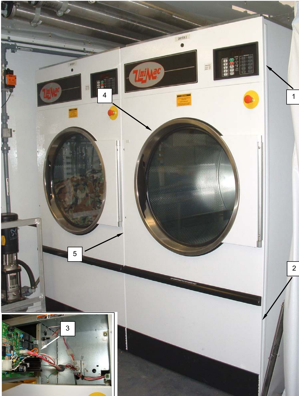
Figure 1. Test the Dryer Emergency Stop Switch.
